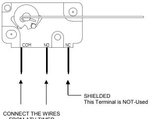
FROM ATV-TIMER TO THE COIN MIRCO-SWITCH "COM" AND "NO" TERMINALS
